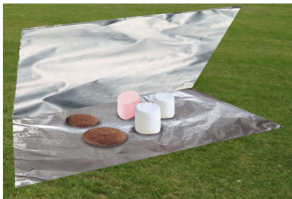
SOLAR OVEN: fold the foil-covered card in half to form the oven base and lid.
